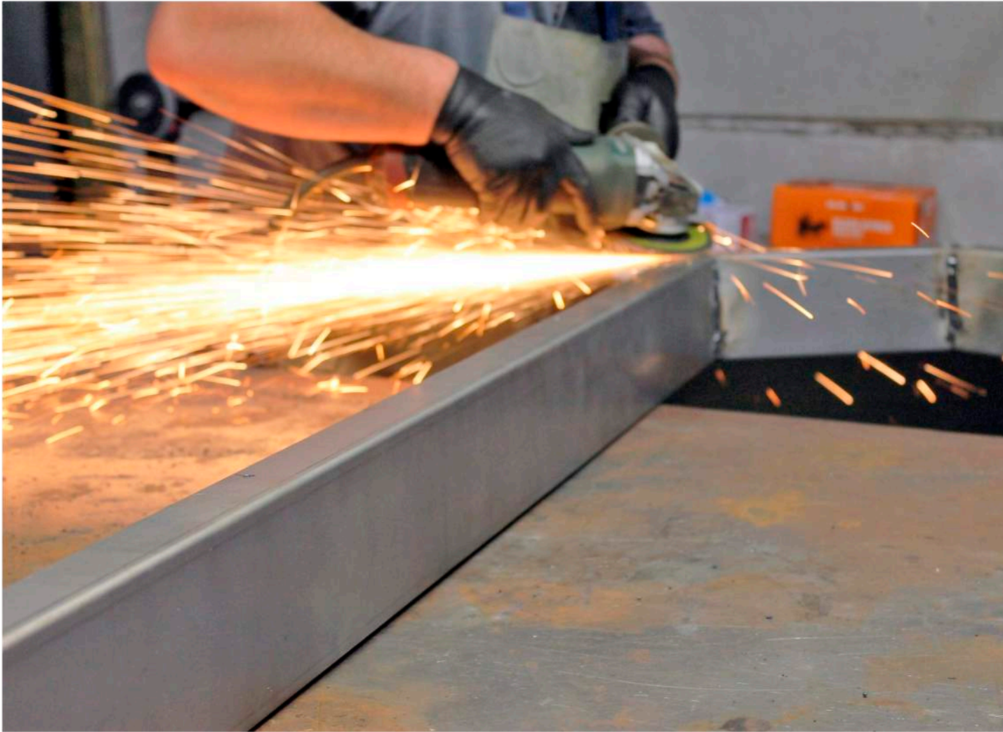
Internal structure. Welding retouching.
