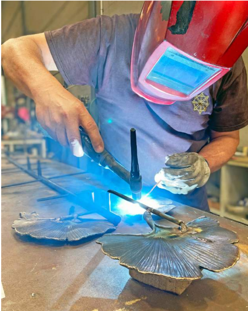
Welding the leaves to a structure previously manufactured.
